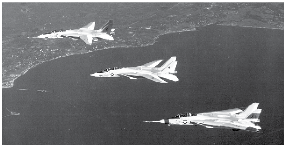
Three F-14A Tomcat prototypes 1972, showing the different wing configurations that were available. (National Naval Aviation Museum)
